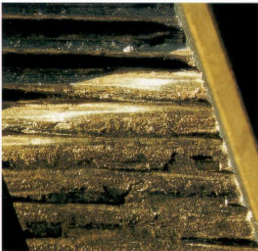
Surface of the rack after resistance test
