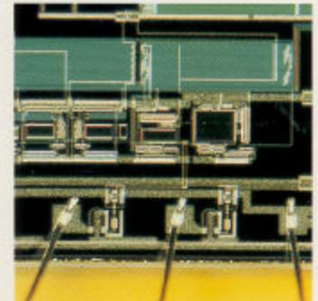
Wire bonding section on the AF sensor
