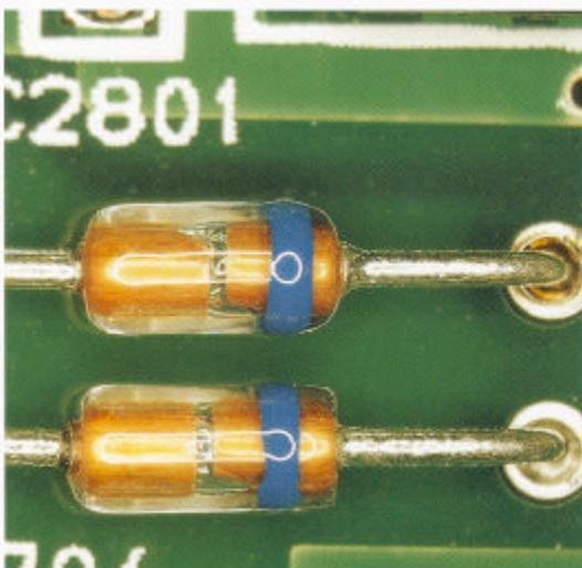
Diode on the circuit board
