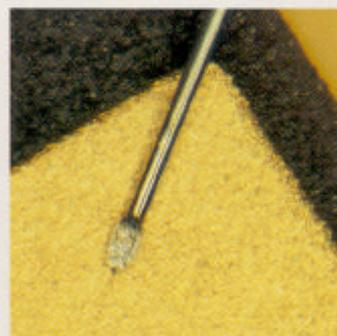
Wire bonding section on the AF sensor
