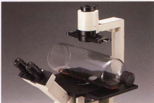
Detachment of condenser provides an ultra-high working space
