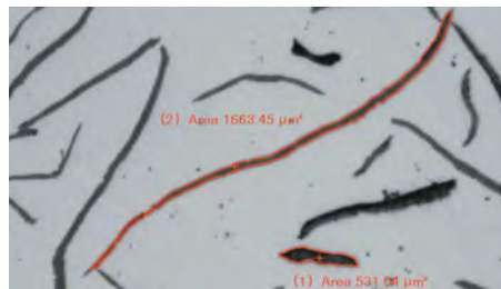
Measurement result using Magic Wand** (cast iron)
