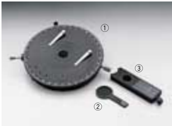
① U-SRG2 rotatable stage ② BX45-PO polarizer ③ U-GAN gout analyzer
